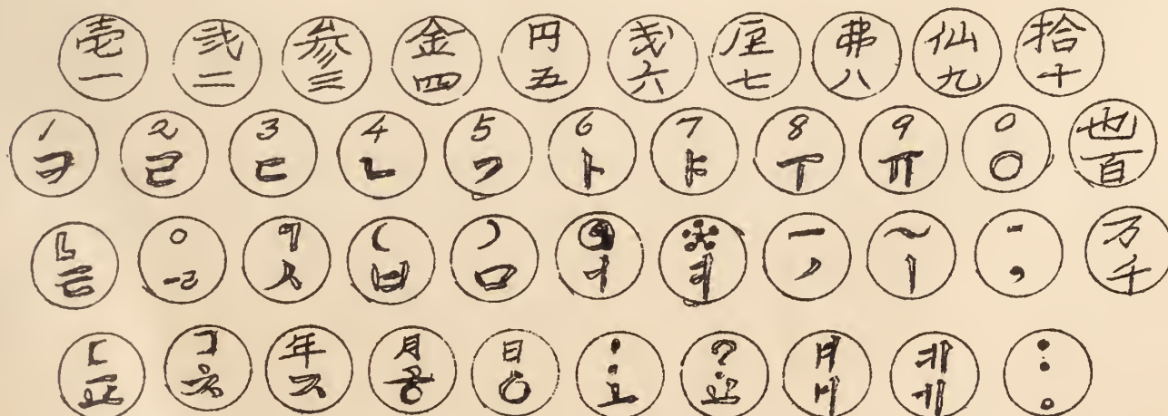
DIAGRAM "B" ( The Keyboard of the New Korean Typewriter ):
